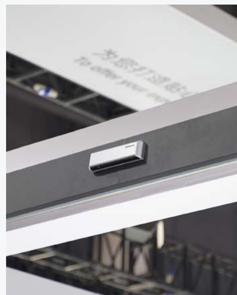
Infrared radar for detecting pedestrians and automatically opening.
